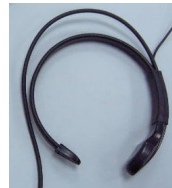
VOX activated by skin(throat) vibration
